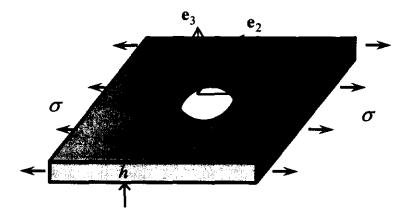
direction), but there is a stress concentration at A (i.e.  $x_1 = 0$ ,  $x_2 = d/2$ ,  $x_3 \in [0,h]$ ) of 3:  $\sigma_{11} = 3\sigma$ . This will change when  $\sigma$  becomes large enough to trigger plasticity.
