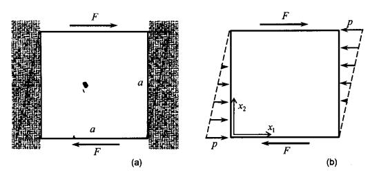
In order to compute the peak value p of this distribution, the principle of virtual work is adopted with the virtual displacement field given by
